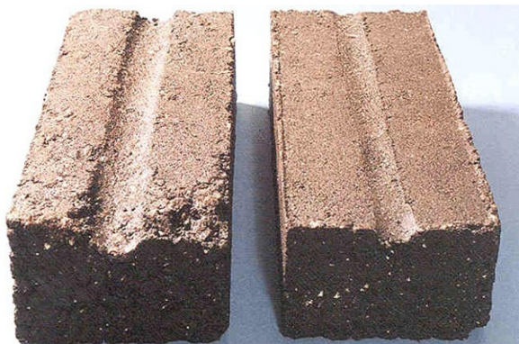
Fig. 6.7 Rutting depth of the HMA prism specimens with and without slag.
