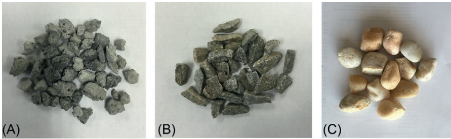
Fig. 12.1 Comparison of the texture and particle shape of different aggregates for concrete. (A) Electric arc furnace slag; (B) crushed stone; and (C) gravel.
