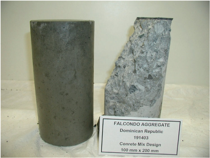
Fig. 12.12 Concrete containing nickel slag aggregate after compressive strength testing.
