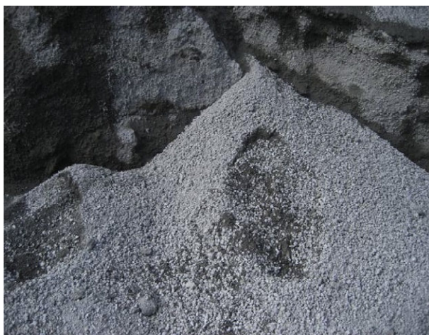
Fig. 11.15 Air-cooled and water-quenched EAF slag from MultiServ-Harsco, Hertford, North Carolina has been used in pervious PCC. The results indicate the PCC possesses good physical and mechanical properties.
