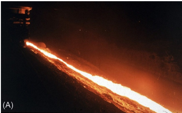
8.4 The dumped molten ferronickel slag is fragmented by “thermal shock.” during ambient cooling in the slag storage area (A).
