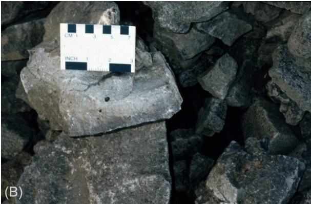
8.4 Continued. Fragmented sized and crushed and screened to a wide range of gradations for highway construction uses (B).
