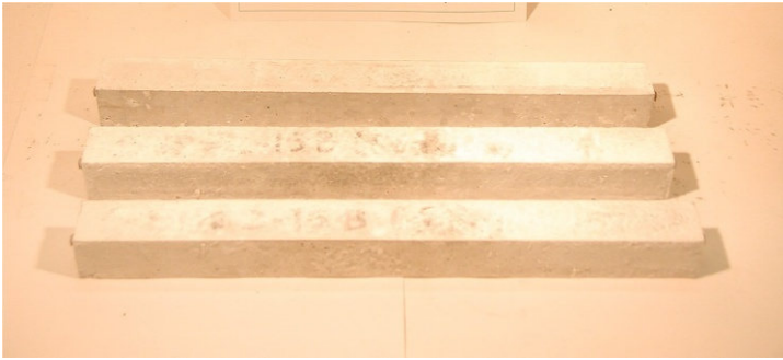
Fig. 11.14 Concrete containing 12.7 mm (0.5 in.) air-cooled nickel slag after a 28-day mortar bar test.
