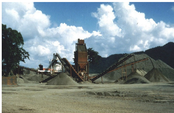
Fig. 14.10 Crushing/screening river gravel to be blended with Falcondo aggregate for subbase and base material.
