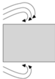
FIGURE 5.3 Vortices on along-wind sides of the building
