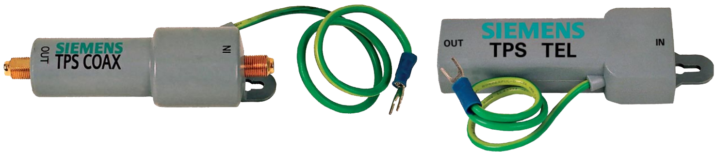
Stand-alone coax (left) and telephone (right) surge suppressors. Note the ground wire: Each must be connected to grounded metal or a grounding pin in a receptacle outlet. Courtesy Siemens Corp.
