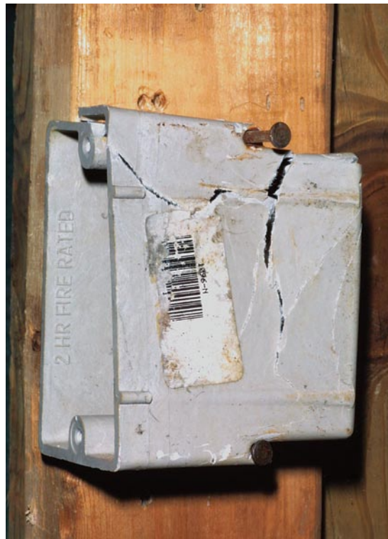
Fiberglass boxes are sturdy but can easily be destroyed by one misplaced hammer blow.
