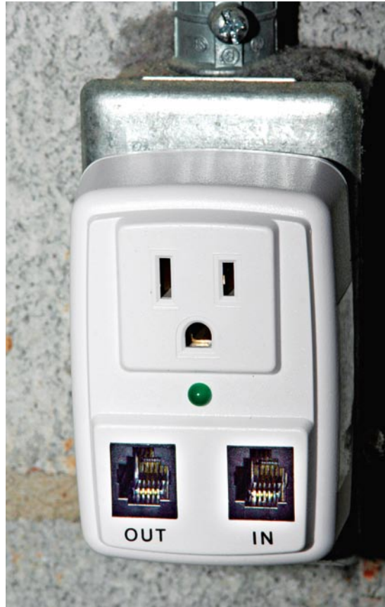
Plug-in type telephone-cable surge protectors are incorporated with a receptacle so they can use the outlet's ground pin and EGC to take away surges.
