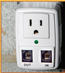
306 | Phone and Coaxial Cable Protection
