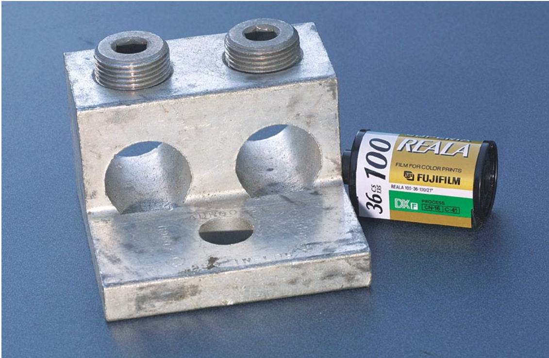
About the size of two 35mm film cartridges, this two-cable lug bolts onto a 400-amp meter base. The lug attaches onto a bus immediately below the meter itself. You'll need three of these (hot, hot, and neutral) if you are installing two 200-amp service panels.
