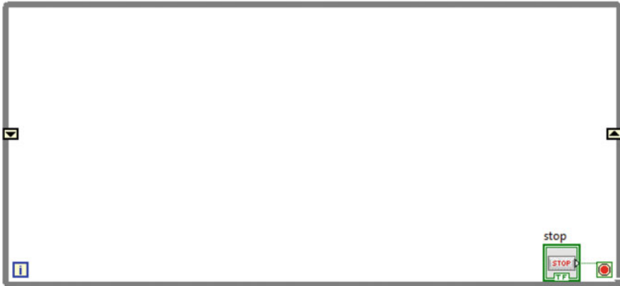
Fig. 14.2 While-loop with a shift register. Rightmost is current value we send data to, left is past values we retrieve data from
