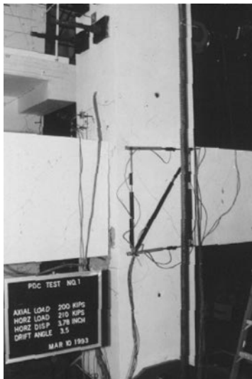
Figure 2.1.66 Condition of the test subassembly of Figure 2.1.64 at a drift angle of 3.5%.
