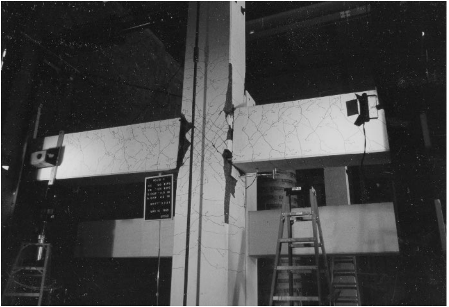
Photo 2.7 Beam-column joint—test specimen, University of California San Diego.
