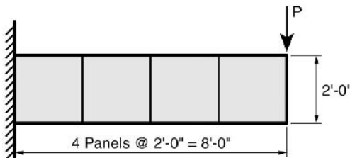
Figure 1.3.11 Beam shear deflection model.
