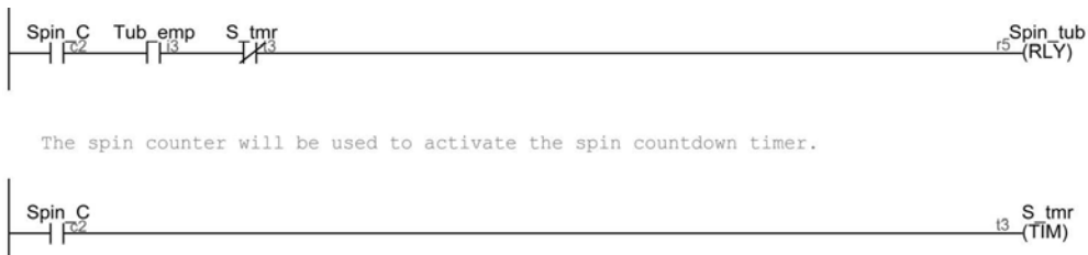
Figure 9-75 Spin tub state transition logic
