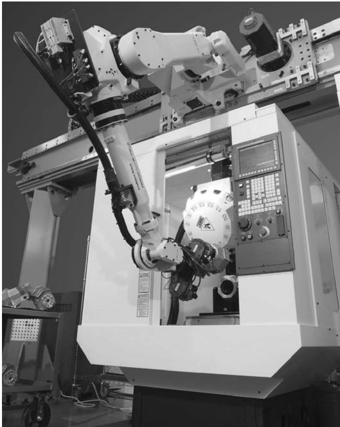
Figure 6-24 Robot machine loading and unloading
