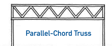
Parallel-Chord Truss PARALLEL-CHORD TRUSSES ARE FOR FLAT ROOFS; STANDARD SPANS ARE AVAILABLE UP TO 30 FT.
