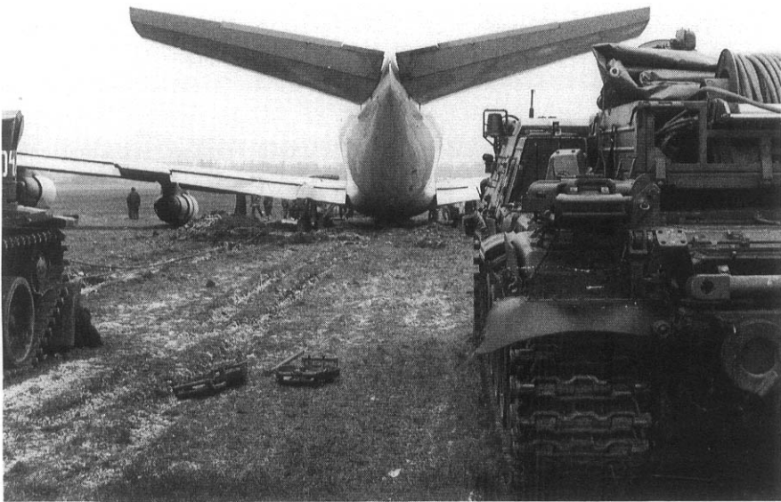
Figure 13-4 The airplane recovery after runway end overrun, photo: J. Mach
