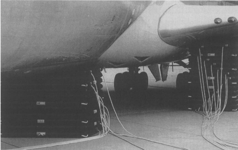
Figure 13-6 Lifting of aircraft by special air bags
