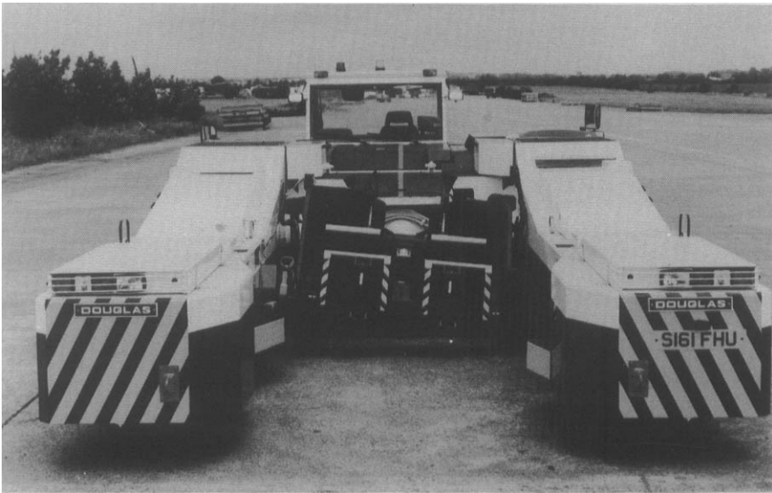
Figure 8-7 Douglas TBL 400 Towbarless tractor (photo courtesy Douglas)
