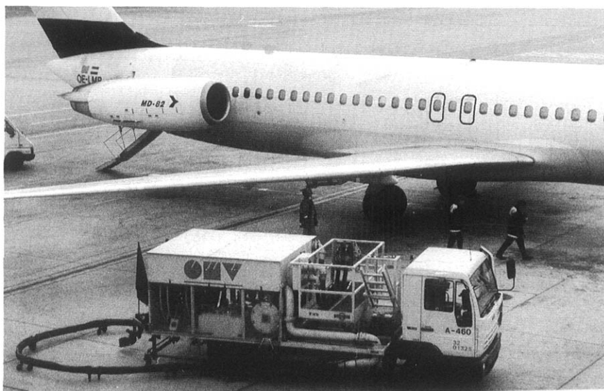
Figure 9-2 Aircraft refuelling by fuel dispenser (photo A. Kazda)
