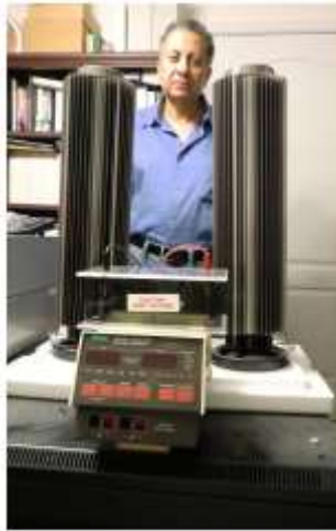
Figure 8. Electrophoretic deposition equipment used by the author.
