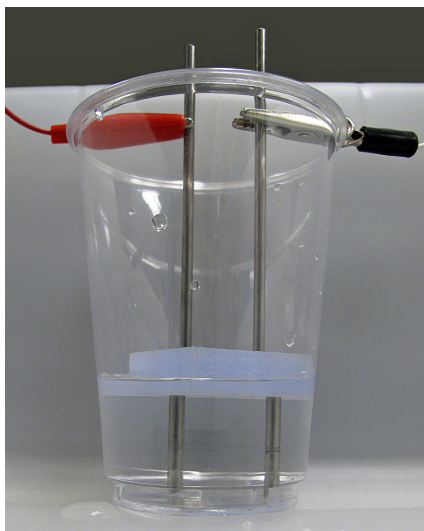
Figure 39.2: Stainless-steel electrodes made from 1/8" 316L stainless-steel TIG welding rod, showing proper depth for immersing electrodes to get repeatable surface area and use of alligator clips to stabilize the electrodes in the cup.
