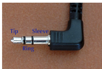
Figure 31.1: A TRS (tip-ring-sleeve) plug for earbuds or other stereo audio applications. The tip is the left channel, the ring is the right channel, and the sleeve is ground.
