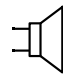
Figure 29.3: The schematic symbol for a loudspeaker is intended to be physically iconic, with the trapezoid corresponding to the cone and the rectangle corresponding to the permanent magnet and voice coil. The two connections are to the two ends of the voice coil.
