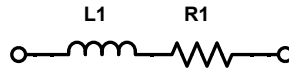
Figure 28.3: We often model actual inductors as an inductance ( L_1 ) in series with the resistance of the wire used to make the inductor ( R_1 ).
