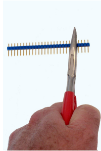
(a) Hold the headers right next to the spot where you want to break them—here they are being held for breaking off four header pins. If you have only one pair of pliers, use your fingers for this first grip.
