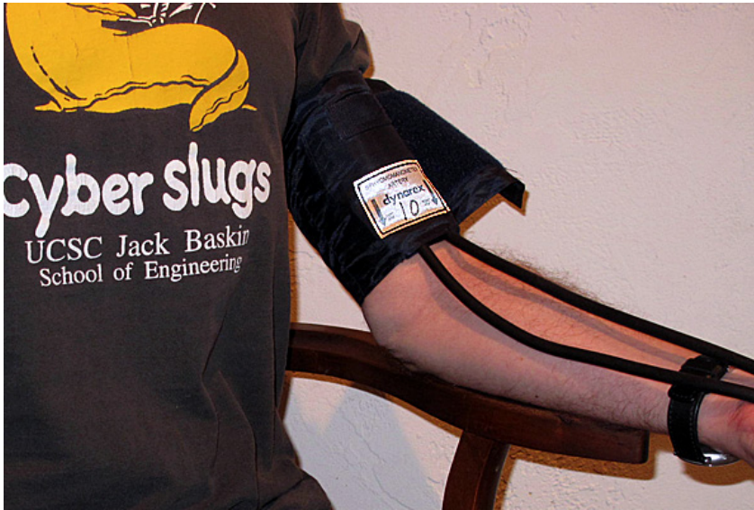
Figure 21.1: This picture shows the correct positioning of the cuff, with the left-arm arrow pointing to the brachial artery, the arm fully supported, and the cuff at the level of the heart.
