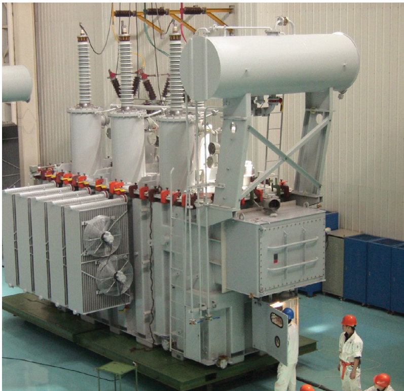
FIGURE 1.17 Large power transformer showing tank and attachments.
