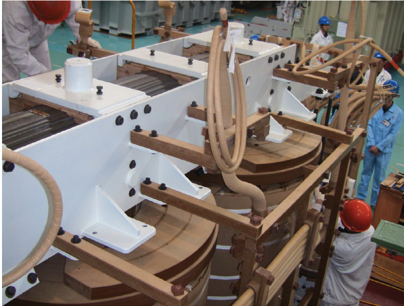
FIGURE 1.16 Top view of clamping structure for a 3-phase transformer.
