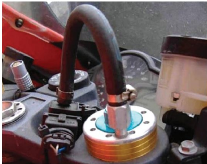
Figure 13.14 Installation of the pressure/temperature sensor on the front shock absorber in a motorcycle
