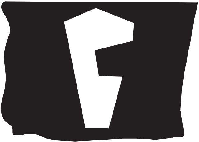
Figure 6.24 Asymmetric rotor slot construction for double-cage machine with good thermal heat capacity.
