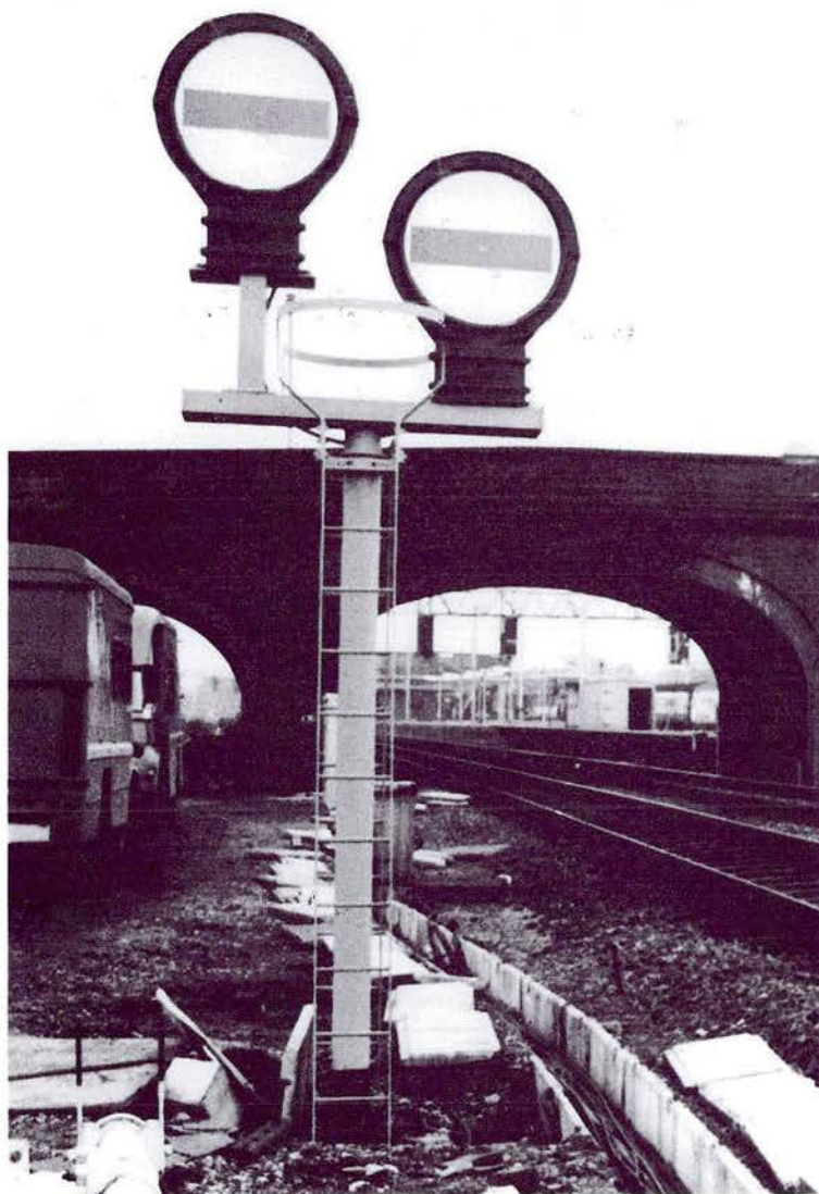
Fig. 7.3 Typical arrangement of banner repeating signals with right hand route (West Hampstead BR-LMR) [photograph by courtesy of Westinghouse Signals Ltd]
