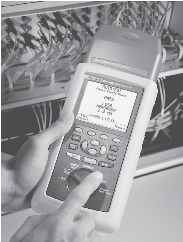
FIGURE 11.14 Fiber cable tester. (Courtesy of Fluke Networks.)
