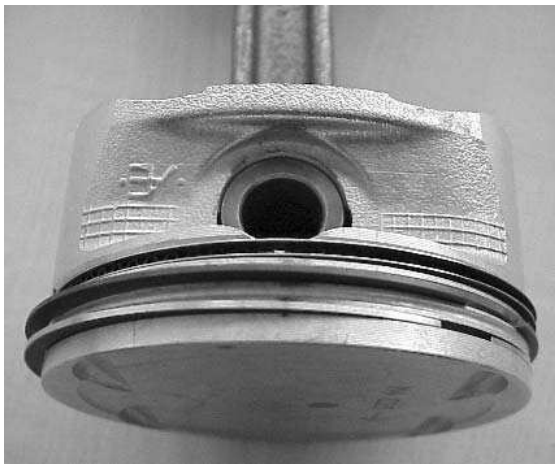
Figure 3.9 Sealing of an internal combustion engine cylinder.
