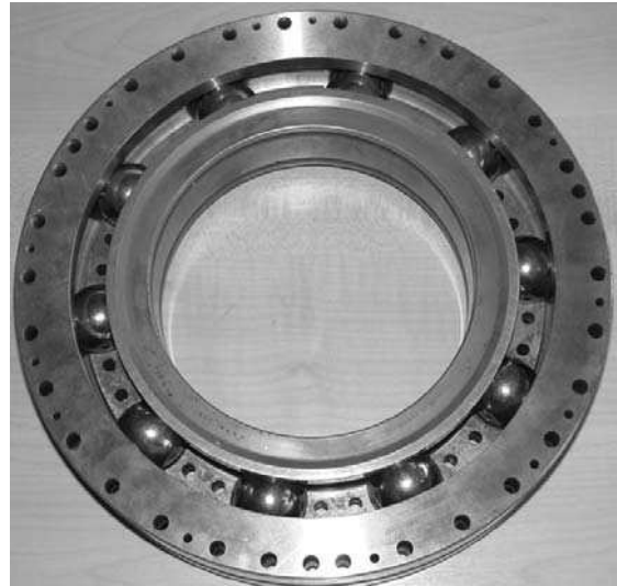
Figure 4.25 Thrust bearing from the Rolls-Royce Trent series of engines.
