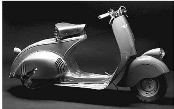
Figure 1.1 Piaggio's Vespa launched in 1946 (Piaggio Museo). The Vespa was an early example of monocoque construction where the skin and frame are combined as a single construction to provide appropriate rigidity and mounting for the vehicle's components and riders.
