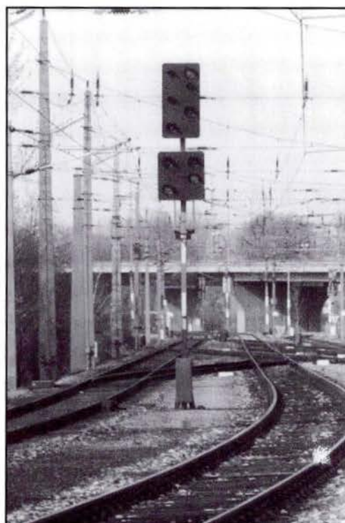
Fig. 4.17 ÖBB: main signal (showing free) with distant signal (indicating next main signal free)
