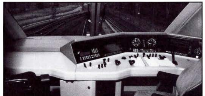
Fig. 7.2 Signal and telecommunications equipment on board a locomotive. Radio equipment on left-hand side
