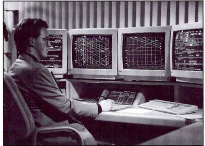
Fig. 11.15 Traffic supervision system (RZÜ), Frankfurt, with four high density monitors, a dialogue monitor and a digitizer. Photo: Alcatel SEL
