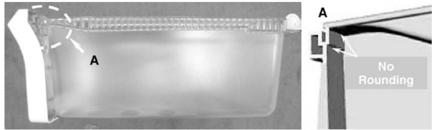
Fig. 8.93 Structure of failing drawer system in field
