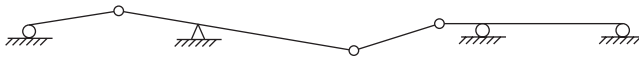
Fig. 12.14 The mechanism (read: collapse) of the bridge if the closing section also had been severely damaged.
