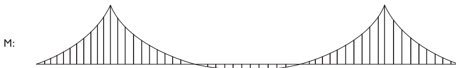
Fig. 4.5 The moment distribution of a continuous girder (or Gerber beam) for self-weight and evenly distributed load. The highest values are found in the negative bending moment region over the two inner supports.
