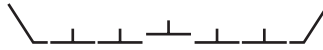
Fig. 17.12 As a simplified approach the longitudinal stiffeners are assumed to buckle independently of each other.
