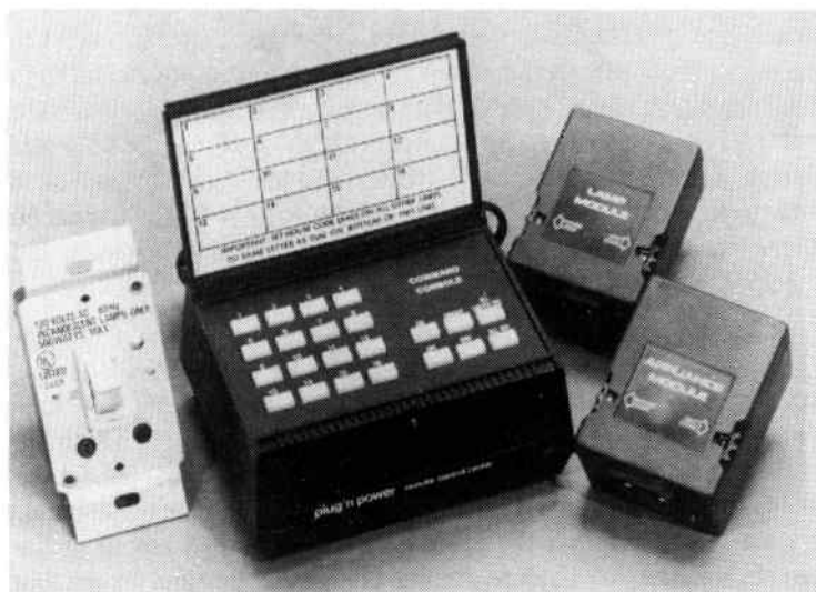
Fig. 10-15. Master and remote models for wireless control of electrical devices.
