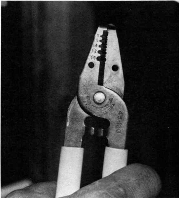
Fig. 6-37. A wire stripper is a handy tool.
