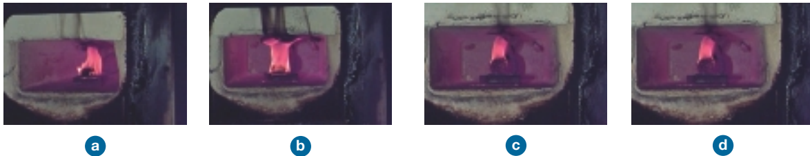
Figure 2.25 Initial stage of combustion of a (a) ignition; (b) 30s; (c) 60s; (d) 120s piece of car tyre rubber in a 900°C furnace
