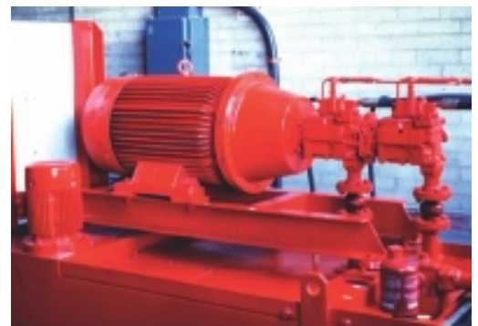
Figure 4.73 Hydraulic power pack showing 75 kW motor and pump, and below them the oil storage tank
