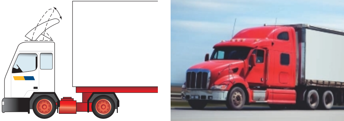
Figure 1.24 A deflector can reduce the pressure drag of a truck by 20%, by steering the streamlines away from the frontal surface of the trailer. If there is no trailer attached to the cab, however, there will be a large increase in drag.
