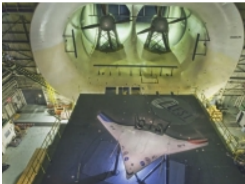
Figure 1.45 Wind tunnel test of the X-48 blended wing body at NASA Langley Research Center
