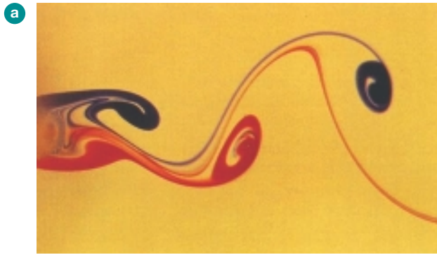
Figure 1.38 Vortex shedding from a circular cylinder. (a) Flow visualization; (b) Strouhal number (non-dimensional frequency for vortex shedding) as a function of the Reynolds number.
