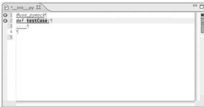
Figure 8-9. The pym template being expanded
