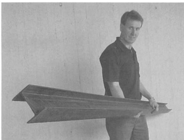
Fig. 5.24 Prototype, structural I-beam, produced using carbon fiber tows and NCFs with an epoxy resin system. Courtesy of CRC-ACS Ltd, Australia.
