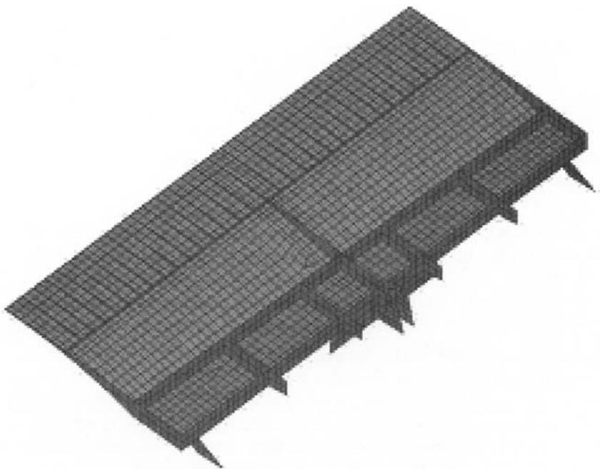
Fig. 16.3 Finite element model for a wing spoiler—top skin removed.
