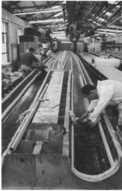
Fig. 15.4 Fiber Bragg grating sensors being embedded in carbon/epoxy composite yacht mast during construction. 10
