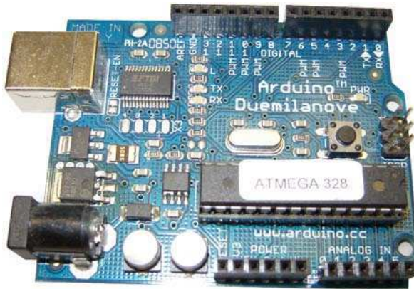
Fig. 4.1 Arduino Duemilanove Board Based on the ATmega168/ATmega328 Microcontroller
