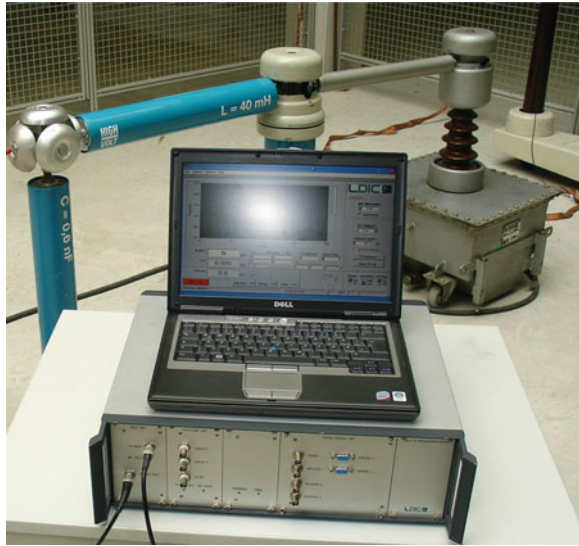
Fig. 4.27 View of a digital PD measuring system (Courtesy of Doble Lemke)
