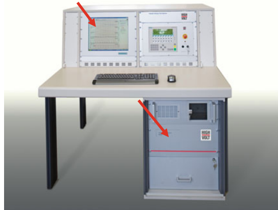
Fig. 2.11 Instruments for HV measurement. a Digital AC/DC peak voltmeter. b LI/SI digital recorder
