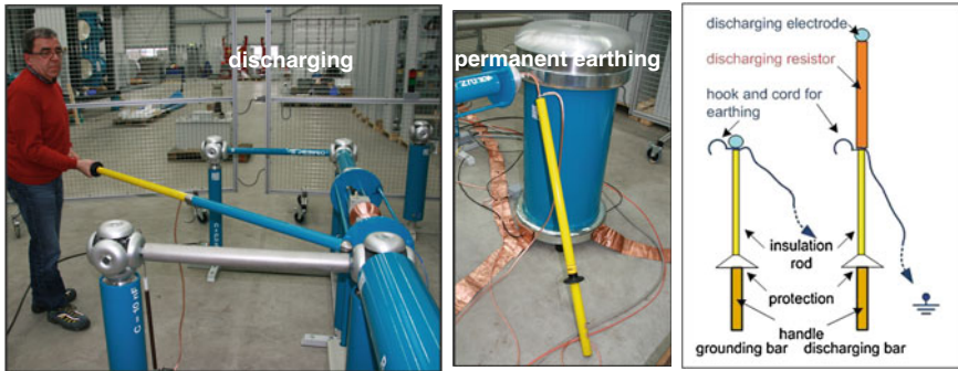
Fig. 6.14 Grounding of smaller HVDC generators
