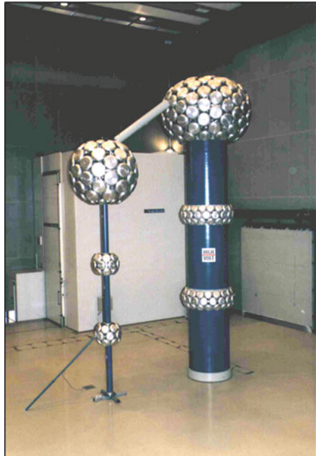
Fig. 3.10 Cylinder-type test transformer 500 kV/500 kVA. a Complete transformer. b Active part with divided windings
