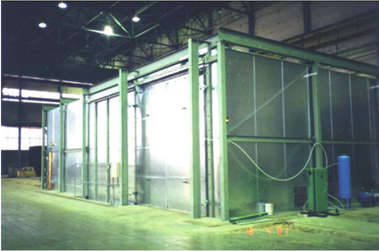
Fig. 9.32 Shielded cabin in a routine test field
