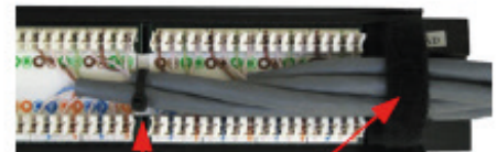
Insulation Displacement Connector (IDC) Punch Down Strip
