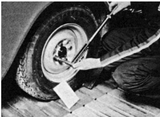
Fig. 8.30 Using a torque wrench for the final tightening
