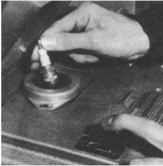
Fig. 11.64 A spark plug cleaning machine
