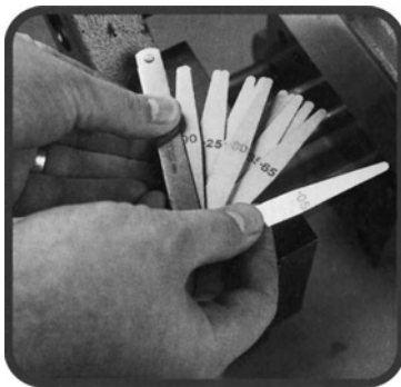
Fig. 13.2 A set of feeler gauges. (Reproduced with the kind permission of Bowers Metrology Group.)
