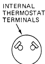
Fig. 7-48 Glass quick-connect terminals for Au and AR models. (Tecumseh)
