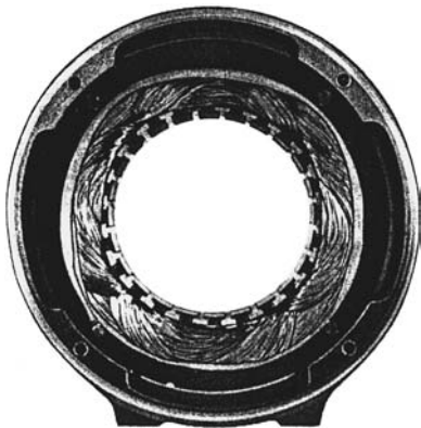
Fig. 5-19 Split-phase motor windings. (Bodine Electric Co.)
