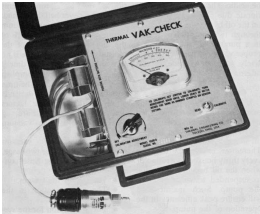
Fig. 1-57 An electronic high-vacuum gage that reads directly in microns. (Thermal Engineering)
