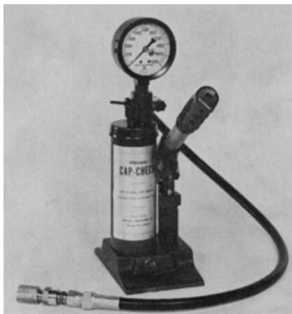
Fig. 1-50 Cap-Check is a portable self-contained hydraulic power unit with auxiliary equipment that is especially adapted to cleaning refrigeration capillary tubes. It is hand operated.
