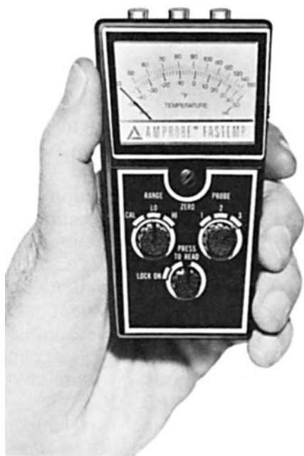
Fig. 1-32 Hand-held electronic thermometer. (Amprobe)
