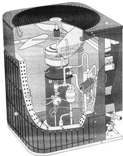
Fig. 7-83 HP-20 Model with a heavy-duty scroll compressor. 1, cabinet; 2, coil area; 3, copper tubing; 4, fan; 5, scroll compressor. (Lennox)
