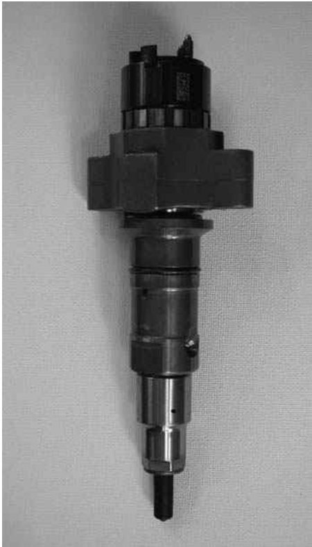
Figure 13-2 External view of an EHI used in a modern CR-fuel system.
