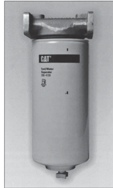
Primary filters on modern engines are typically rated at 10–15 microns
