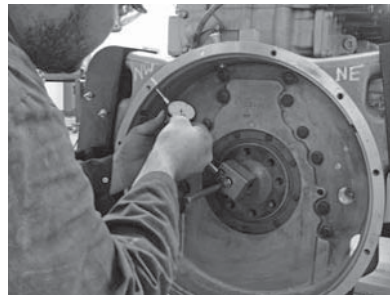
P3-5 Now fit a dial indicator with a magnetic base at any secure location on the crankshaft. Choose one of the four reference points and zero the indicator to it. Here we have chosen to begin at the NW reference location.
