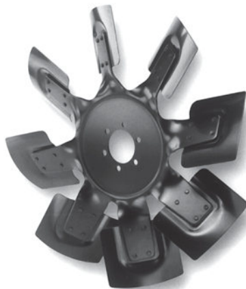
Figure 8-14 Various diesel engine fan blades used in current trucks. (Courtesy of Horton)
