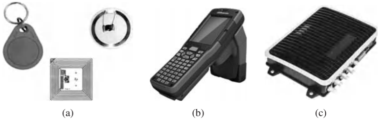
Figure 5.15 (a) Examples of RFID tags; (b) a portable RFID reader; (c) a fixed RFID reader.
