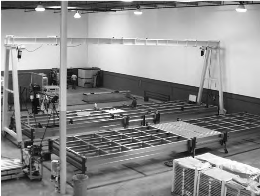
Figure 2.12 Amonix MegaConcentrator platform assembly.
