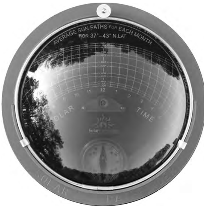
Figure 4.14 Pathfinder dome showing solar platform site shading.
