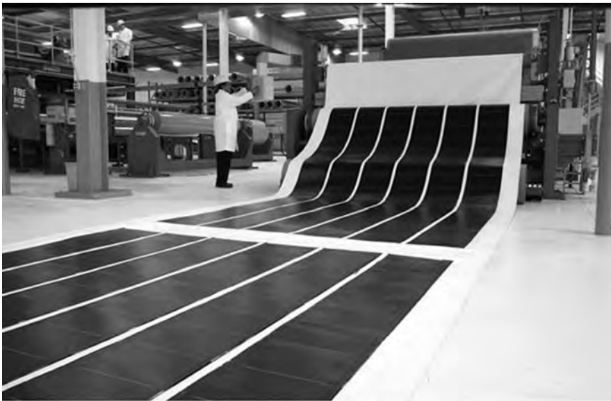
Figure 2.13 Manufacturing process of film technology and single-ply PVC lamination process. Photo courtesy of Solar Integrated Technologies, Los Angeles, California.
