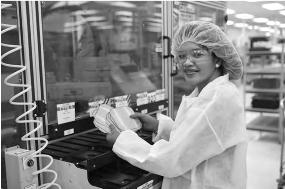
Figure 2.5 Fabricated monosilicon solar cell inspection.
