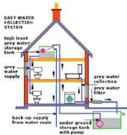
Figure 11.27 Greywater reuse system.
