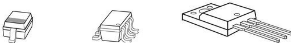
Fig. 11.7 : Diode packages: SOD-323 SMD package (left), SC-74 SMD package (mid), TO-220 THD package (right). Package drawings by Infineon Technologies AG.
