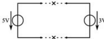
Fig. 3.7: Do not connect ideal voltage sources in parallel.
