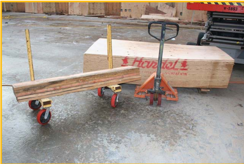
Pallet jack and drywall cart for moving lumber
