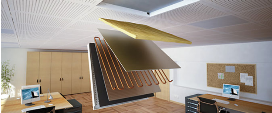
Fig. 5.7 Chilled ceiling panel components (SGL Carbon 2012)
