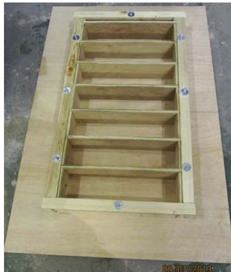
Figure 6.1 Reusable plywood mold for seven specimens.
