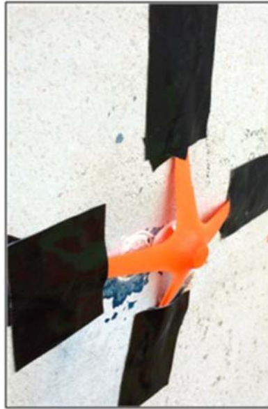
Figure 7.1 Test dolly secured with rubber membrane.
