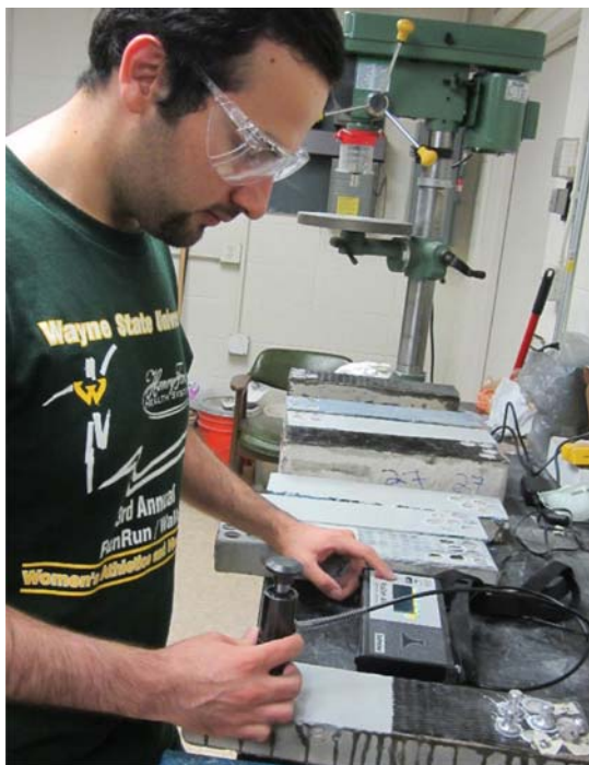
Figure 6.6 Pull-off test underway.
