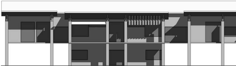
Figure 4.4 View of external shading devices sized in Autodesk Revit Architecture
