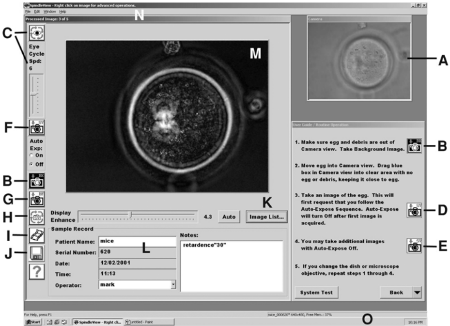
Fig. 2. A full-screen view of the SpindleView software. (A) Camera View (Live Video) window; (B and B') take Background icon; (C) Eye Cycle icon for viewing the spindle through the eyepieces, and Eye Cycle Speed Setting. (D and D') take SpindleView Image icon to take single processed image; (E) take image icon with auto-expose off; (F) display Enhance Control; (G) take Brightfield Image icon; (H) SpindleView Cycle icon; (I) take Timelapse Image icon; (J) save Image icon; (K) Image List icon; (L) Sample Record window; (M) Active Image window; (N) menu bar; (O) status bar.
