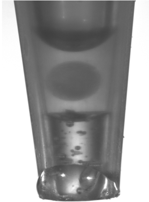
Fig. 2. Homogenizing vessel containing a single unfertilized zebrafish egg. An egg positioned in the homogenizing vessel made from an epoxy-plugged blue 1-mL pipet tip is easily visualized under a dissecting microscope. The water surrounding the egg is removed just prior to homogenization.
