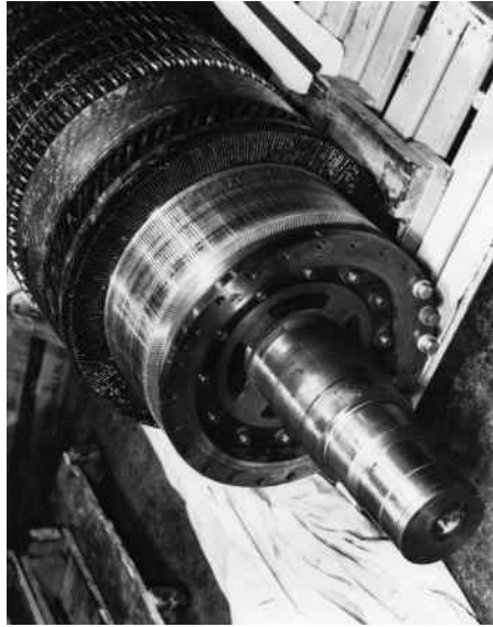
FIGURE 8.6 A close-up view of the commutator of a 500 hp dc motor. (Courtesy of MagneTex, Inc., Menomonee Falls, WI.)
