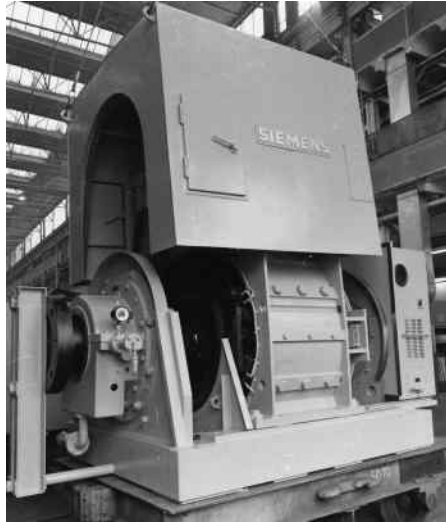
FIGURE 8.1 Mounting the housing of a dc mill motor. (Courtesy of Siemens, Munich, Germany.)
