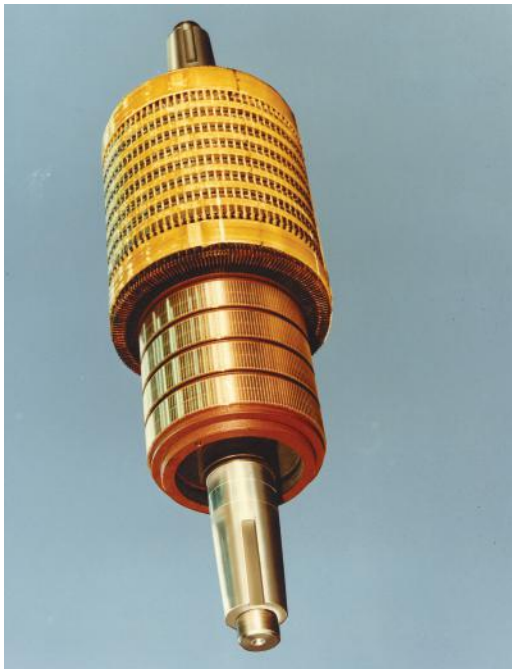
FIGURE 8.7 The armature of a 500 V, 150 hp dc motor. (Courtesy of General Electric, Fairfield, CT.)
