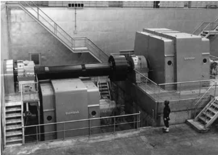
FIGURE 5.6 A dc 8 MW, 50/100rpm dc reversing mill motor operating at 899 V. (Courtesy of Siemens, Munich, Germany.)
