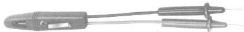
Fig. 19-2 This inexpensive neon test light can be used on either 120-volt or 240-volt circuits and is also handy for testing fuses. It contains a tiny neon bulb that consumes only the smallest fraction of a watt and lasts many thousands of hours. (A. W. Sperry Instruments Inc.)
