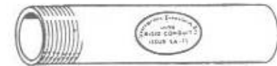
Fig. 12–1 Rigid metal conduit looks like water pipe but differs in several important aspects. It comes only in 10-foot lengths and each length bears a UL label.
