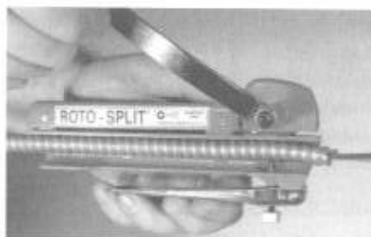
Fig. 11-9 A cable cutter offers the safest and quickest method of cutting armored cable. (Seirek Co., Inc.)
