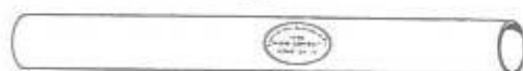
Fig. 12-5 EMT cannot be threaded. It is much lighter than rigid conduit. It comes only in 10-foot lengths.
