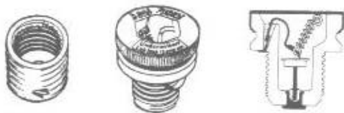
Fig. 5-3 A typical Type S nontamperable fuse (center, and cross section at right) and its adapter (left). Once an adapter has been screwed into a fuseholder, it cannot be removed. This prevents the use of fuses larger than originally intended.
