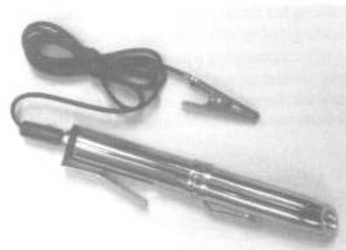
Fig. 11-7 A continuity tester. Use only on de-energized circuits. It is also handy for testing fuses. (A.W. Sperry Instruments, Inc.)
