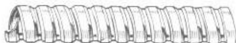
Fig. 12-8 Flexible conduit is installed in the same way as armored cable, but wires are pulled into place later.
