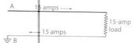
◀ Fig. 10-13 One 2-wire, 120-volt circuit carrying 15 amps.
