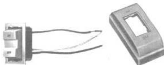
Fig. 18-5 The type of switch used in remote-control wiring is shown above. The same kind of switch is used at every location. It is equivalent to two push buttons. Use as many switches as you wish to control one outlet (or several outlets if you wish). (General Electric Co.)
