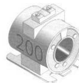
Fig. 17-3 A current transformer.
