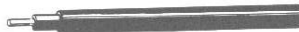
Fig. 17-5 Type USE cable is designed to be buried directly in the ground without further protection. It is available also as 2-wire or 3-wire cable.
