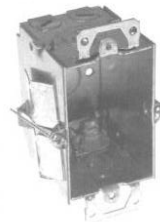
Fig. 13-6 This box has exterior collapsible clamps on each side. Push box into opening, tighten screws on sides, and the box will be anchored in the wall. (Hubbell Electrical Products)
