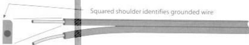
Fig. 4-7 In Type SPT-2, the wires are embedded in plastic. The cord is durable and attractive.
