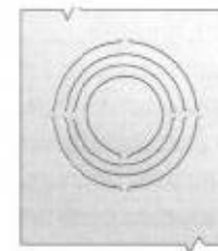
Fig. 8-22 Concentric knockouts are convenient, but great care must be used in removing each section.
