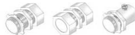
Fig. 12-6 A compression connector and coupling (left and center) used with thinwall conduit. The connector on the right, by comparison, uses a setscrew instead of a compression ring to secure the tubing.
