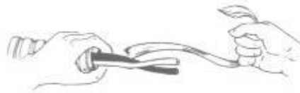
Fig. 11-14 A sharp yank tears off the paper inside the armor, and makes room for the anti-short bushing.
