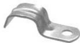
Fig. 8-16 Entrance cable must be anchored to the building every 30 inches. Use straps of the type shown. (The Halco Company)
