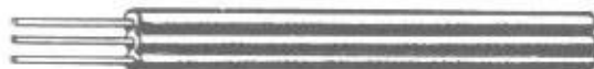
Fig. 18-6 There are only 24 volts on the control wires in remote-control wiring, so inexpensive wire is used. However, it must still be suitably listed because it is a potential fuel load in a fire.
