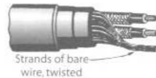
Fig. 8-13 When using the cable, the separate strands of the neutral bare wire are gathered into a bunch making one large wire.
