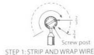
STEP 1: STRIP AND WRAP WIRE
