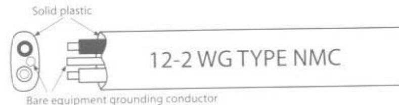
Fig. 4-5B Nonmetallic-sheathed cable, Type NMC, may be used in dry or damp locations.
