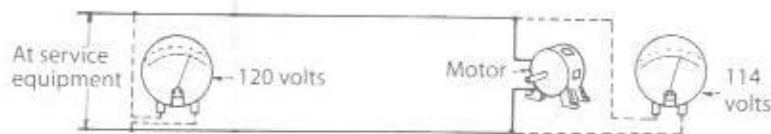
Fig. 4-2 Circuit showing voltage drop—voltage at motor is lower than at starting point.
