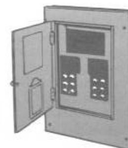
Fig. 8-5 A 100-amp switch. Besides main fuses, it has plug fuses for twelve 120-volt circuits, and cartridge fuses for two 240-volt circuits. ▶
