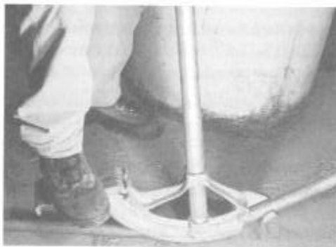
Fig. 12-2 A conduit bender, and method of use. This one bends 1-inch rigid or intermediate metal conduit, or 1\frac{1}{4} -inch EMT. For best results, use the heaviest foot pressure you can manage. This bender has a hinged, two-position foot pad allowing heavy, straight-down foot pressure throughout the bending process.
