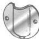
Fig. 8-17 Use a sill plate packed with sealing compound where cable enters building. It keeps water out.
