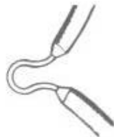
Fig. 4-17 In raceway wiring, a continuous wire may be connected to a terminal as shown here.
