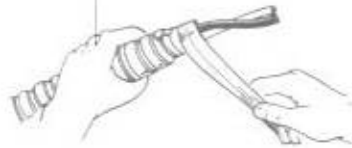
Fig. 11-13 In removing the paper, first unwind a few turns inside the armor.
