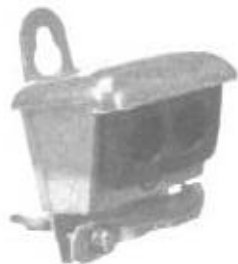
Fig. 8-18 This service head is for cable. It prevents water from entering the cut end of the cable. A service head for conduit is supported by the conduit. (The Halco Company)
