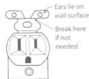
Fig. 15-3 Plaster ears are helpful in aligning a device flush with the wall surface.
