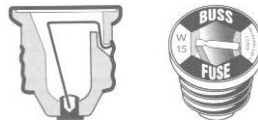
Fig. 5-2 Edison-base plug fuses are made only in ratings up to 30 amps. They are not permitted in new installations.
