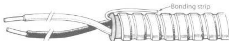
Fig. 11-8 Armored cable consists of 2 or 3 wires protected by a layer of tough paper and flexible aluminum or galvanized steel armor. Note the bonding strip under the armor.
