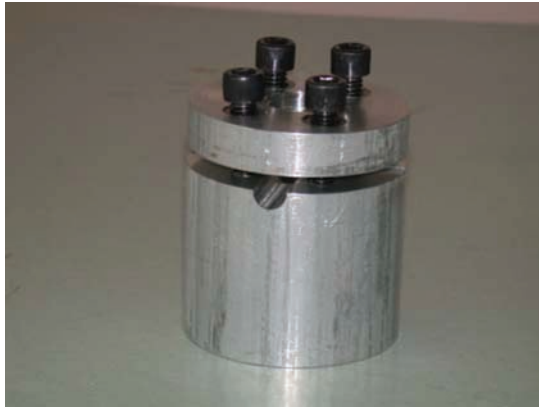
Fig. 4. Special piece used to machine pin on lathe.
