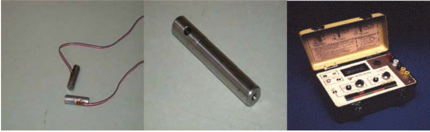
Fig. 3. Pins with strain gages, shaft and P3500 instruments used to measure the strain.
