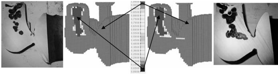
Fig. 4. Shrinkage defect in real and simulated valve ball casting: T_{\text{ini}} = 1257 , S = 2\% , f_1 = 0.1 , f_2 = 0.3 (left) and T_{\text{ini}} = 1307 , S = 2\% , f_1 = 0.1 , f_2 = 0.3 (right).
