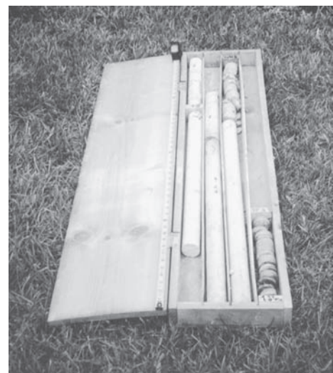
FIGURE 3-5 Core box containing rock core samples.
