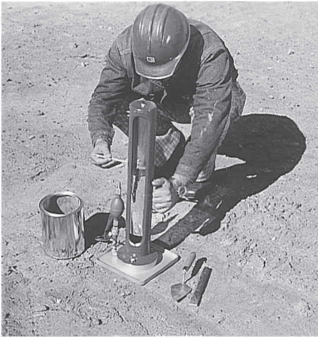
FIGURE 4-13 Rubber-balloon apparatus for determining unit weight of soil in-place.
