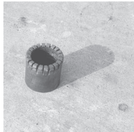
FIGURE 3-4 Cutting bit for rock coring.
