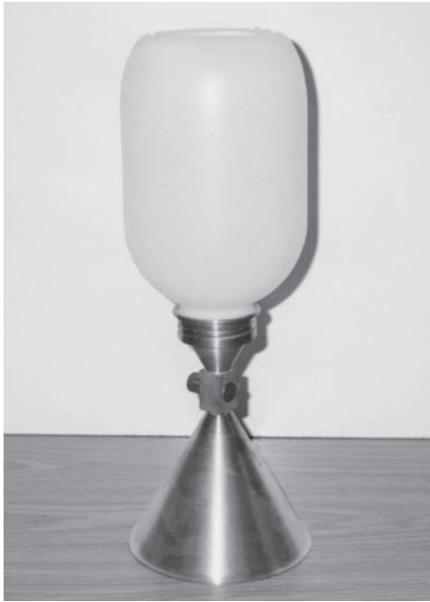
FIGURE 4-11 Density apparatus used in the sand-cone method.
