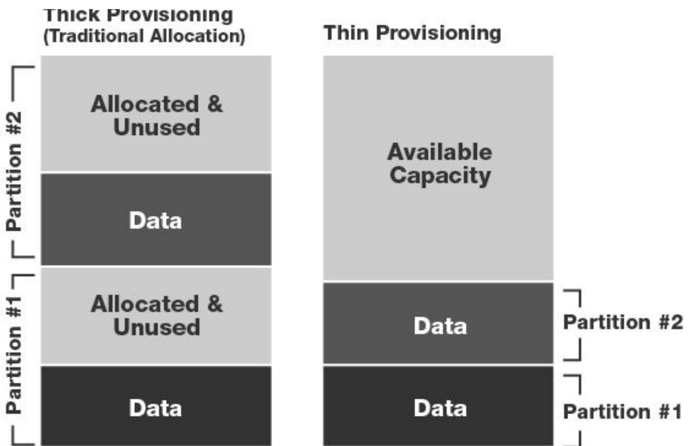
Figure 7-5: Traditional Allocation vs. Thin Provisioning
