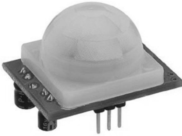
Figure 9-8. Parallax IR sensor
