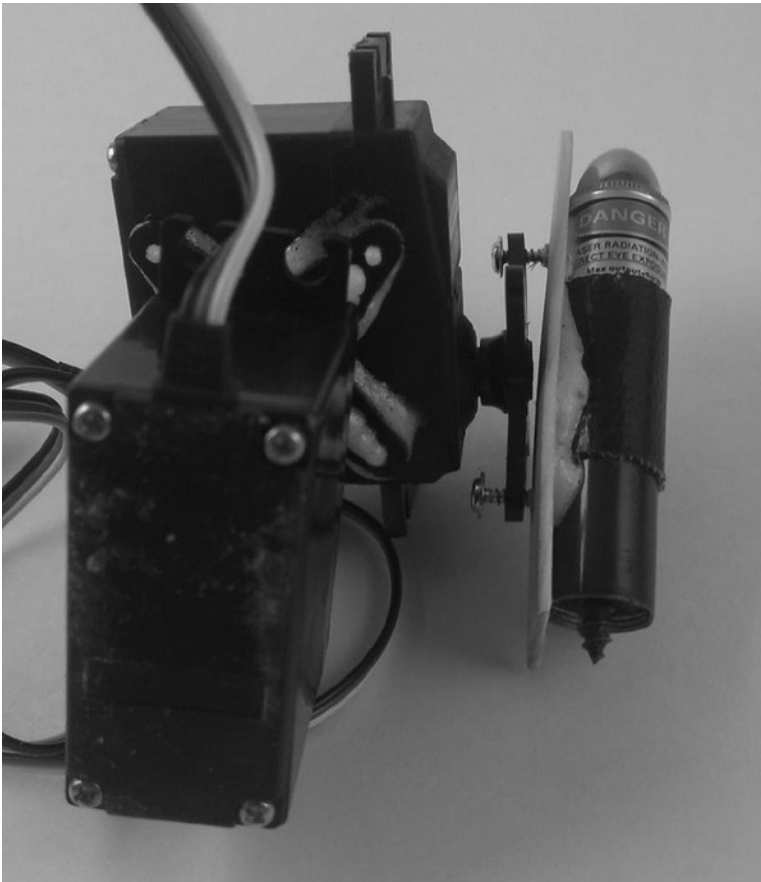
Figure 9-7. Laser mounted to servos
