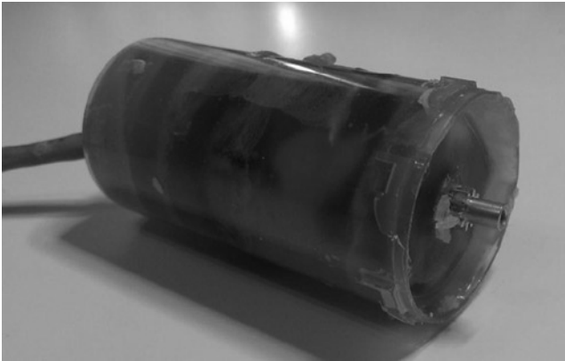
Figure 12-14. Motor surrounded by wax
