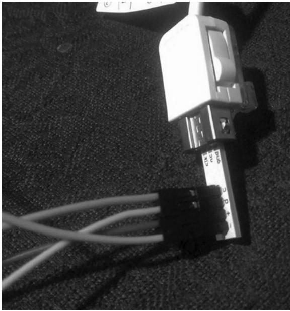
Figure 12-5. Correct positioning of Wiichuck adapter
