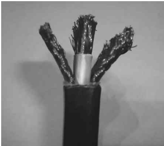
FIGURE 7.11 Virtually concentric Litz cable for 20-kHz power distribution for space station. (Courtesy of M.R. Patel, NASA Report CR-175071, 1986.)
