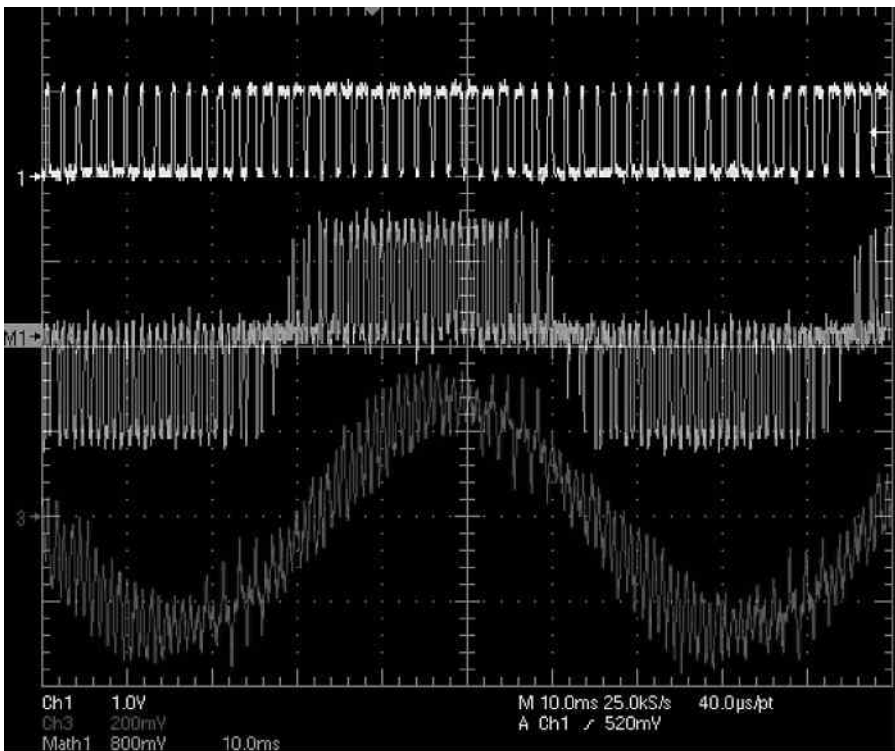
FIGURE 14.11 High-frequency harmonics in PWM converter. (Courtesy of Bill Veit, U.S. Merchant Marine Academy.)
