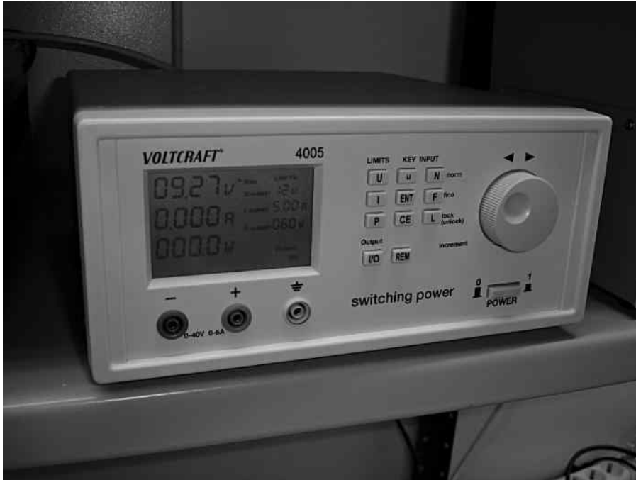
FIGURE 13.14 Switchmode power supply exterior view (Voltcraft 4005). (Courtesy of Nuno Nogueira, Wikimedia Commons.)
