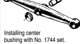
Installing center bushing with No. 1744 set.
