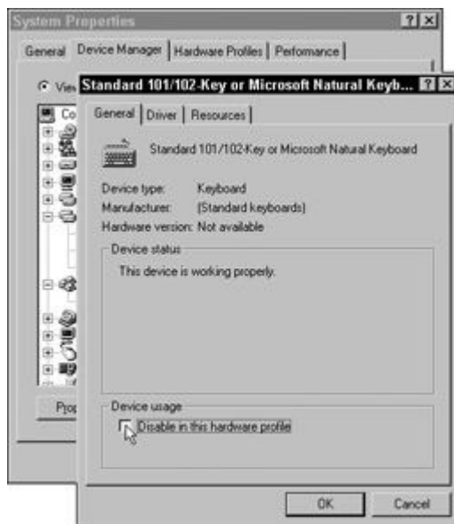
Figure 20-4: The Disable in This Hardware Profile check box is used to disable a device in Device Manager to isolate hardware problems on a Windows system
