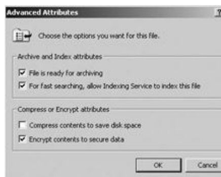
Figure 21-2: The Advanced Attributes dialog box is used to encrypt and compress a file on a Windows 2000 system.
