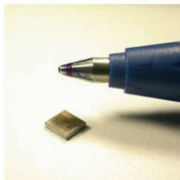
Figure 5. Berkeley “Spec” Mote, 2003
