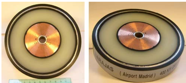
Figure 1.13 Two samples of the “Barajas” Pirelli EHV cable (Courtesy of Prysmian)
