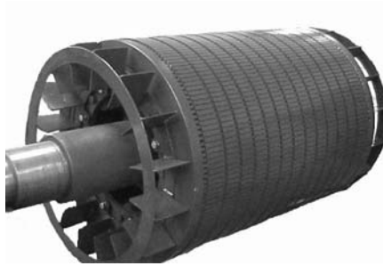
FIGURE 6.3 Finished squirrel cage for large power induction motor (Courtesy of Equacional Motores, Brazil).
